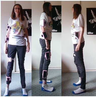
Figure 1: Smartphone placements. The 5 phones are placed on dominant lower arm (outside), dominant upper arm (outside), thigh (outside), lower leg (outside) and non-dominant side hip.
